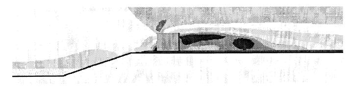
Fig. 1. Simulated hurricane force wind flow over a low residential building structure located downwind of an escarpment.
